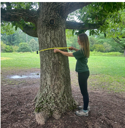
Curatorial Assistant Avery Haislip uses a laser rangefinder (top photo) to measure the height of the tree. Below, she uses a forestry diameter measuring tape to measure the DBH (diameter at breast height) of the tree.
